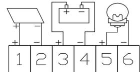
1. Connect the “+”, “-” Poles of the battery to the corresponding ports of controller (the third and the fourth one from left).
